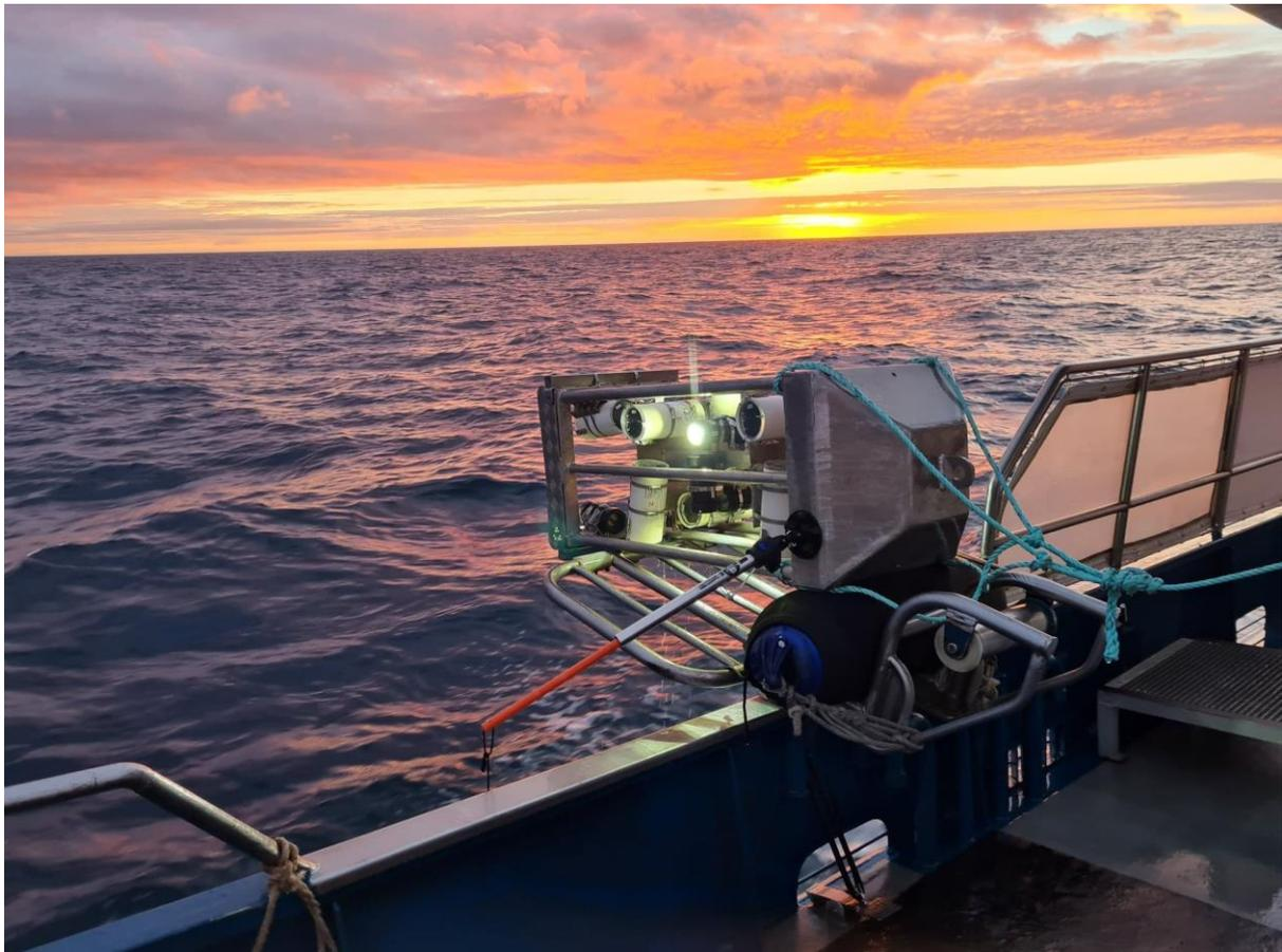
*Figure 5. Panoramic camera laying on side in lobster pot tipper ready for deployment.*
